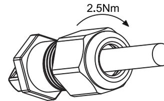
D: Screw the nut tightly with a torque of 2.5Nm.
