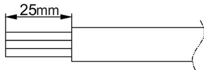
A: Remove the cable jacket for 25mm;
